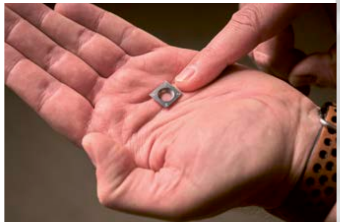
Clean edges without rework: The scraper with a chamfer to prevent material fracturing from LEUCO ensures a uniform finish at Stöcklin Möbel AG and removes visual residues directly during the process.
