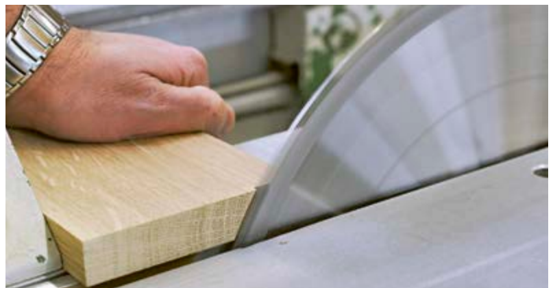
g5-System in use: Cross-cut oak without tearout on the underside
