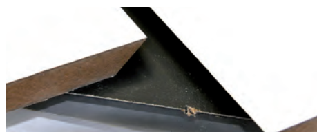
The nn-system saw blade (shown on the left) does not allow any melamine coatings to flake off, ...
