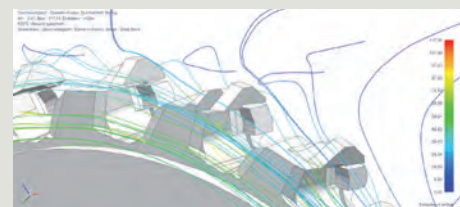
The LowNoise design is visible from first glance: The chip gullets and projecting edges are aerodynamically rounded and optimized with software computations.
