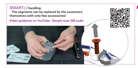
Tip: Given that the tooth rows are subjected to different wear situations, it is possible to replace tooth rows already worn from cutting the top layer with rows from the core layer. Depending on the jointing quality requirements, this method can be useful to prolong the edge life. Of course, you will find all the information needed for proper segment replacement in the operating instructions supplied with the tool.
